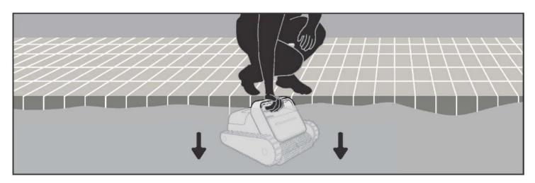
3. Release the cleaner. It takes about 1-2 minutes to complete the self-test and start the cycle.
