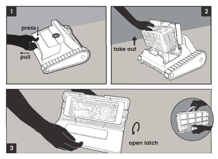
It is highly recommended to clean the filter basket after each cleaning cycle.
