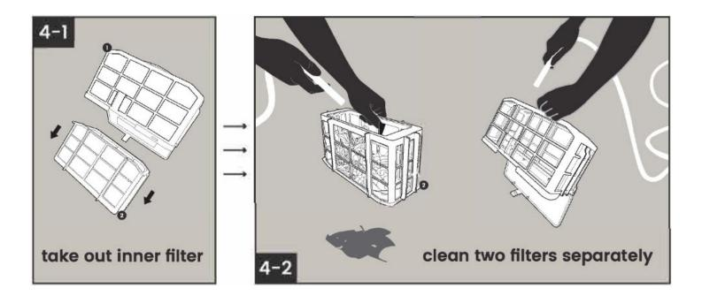
Note: Do not let the filter basket dry out before cleaning. Clogged tilters will affect the overall cleaning performance of your cleaner by making it difficult to create suction or keep dirt and debris in the tilter basket. Replace the tilter basket when the cleaning results are not satisfying and cleaning the tilter does not make a difference.
